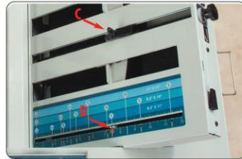
Step 2: Set paper stops by simply sliding the stop levers (C) to match the LED indicator lights (D).
